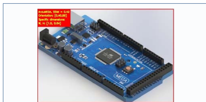
Figure 5: OD on Arduino-MEGA PCB board – isometric view.
