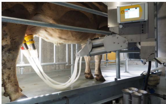
Figure 4: MultiLactor milking machine during milking in a tandem milking parlour according to Kaskous [100].
